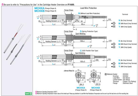
Lead Wire Protection Type with Knurled Flange
