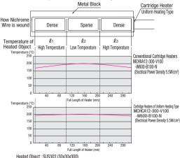
Point of Temperature Measurement: £1, £2, £3 center part of each surface
