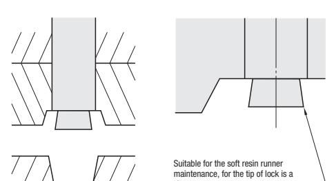
Suitable for the soft resin runner maintenance, for the tip of lock is a sharp corner.
